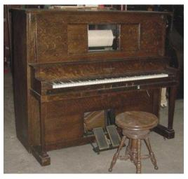
The perforations on a piano roll represent note control data. Air is pumped into the piano by the pedals operated by the player; this can also be done electrically. This air passes through the perforations as the roll turns and is read by the tracker bar which activates the keyboard mechanically. The player piano shown here is a Francis Bacon piano, made by one of the longest running piano builders in America.
